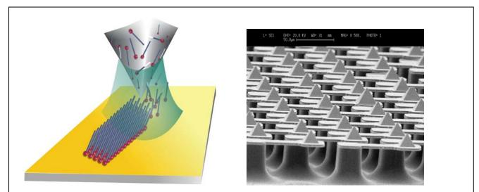
Left: Schematic illustration demonstrating the concept behind dip pen lithography. Right: A portion of a 10,000-pen array used for doing massively parallel dip pen nanolithography (images courtesy of Prof. C. Mirkin, Northwestern University).
