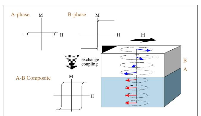
Exchange-Spring Principle for Nanocomposite Permanent Magnets: As long as the length scale does not exceed a magnetic domain wall thickness, the composite behaves likes a single new composite material. When it does exceed this critical length scale, a twist can develop, as shown, in response to a reverse external magnetic field (image courtesy of Samuel Bader, Argonne National Laboratory; reprinted with permission from Rev. Mod. Phys. 78, 1, © 2006, American Physical Society).
