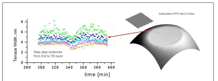
Example of structural fluctuations in the nanoscale features of a micrometer-scale lead crystallite as it approaches its equilibrium shape. The terraces bounding the edge of the crystallite fluctuate with increasing amplitude until just before the nucleation of a new shrinking layer occurs at ~340 minutes (figures courtesy of K. Thürmer, Sandia National Laboratories).
