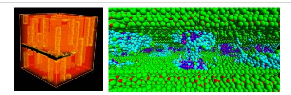
Left panel: Simulation of fractured silicon nitride (red) ceramic reinforced with silica-coated silicon carbide fibers (yellow). Right panel: Close-up of the fractured composite system. Small spheres represent silicon atoms and large spheres represent nitrogen (green), carbon (magenta), and oxygen (cyan) atoms (figures courtesy of R. K. Kalia, A. Nakano, and P. Vashishta, University of Southern California).
