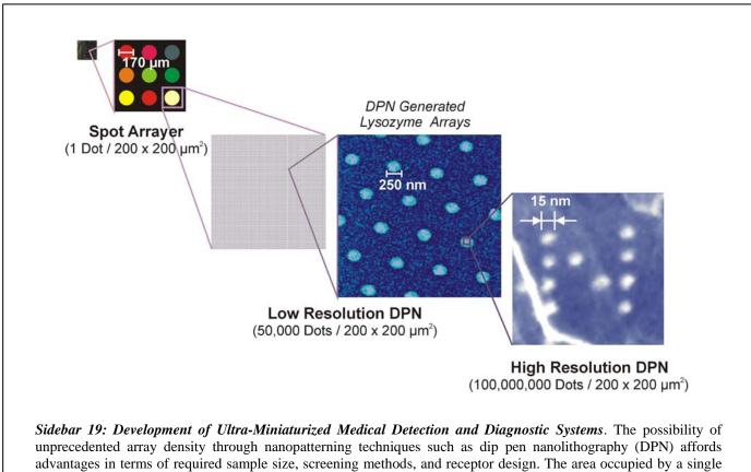
feature in a conventional gene chip based upon conventional microtechnology can be replaced with an entire gene chip or proteomic array with thousands of features (image courtesy of C. Mirkin, Northwestern University).
