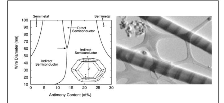
Left: Variation in electronic structure of Bi-Sb nanowires as functions of composition and wire diameter (image from Lin et al., Proceedings of the 21<sup>st</sup> International Conference on Thermoelectronics, 253; reprinted with permission, © 2002, IEEE). Right: Superlattice Ge/Si nanowire (image adapted from Li et al., Appl. Phys. Lett. 83, 3186; reprinted with permission, © 2003, American Institute of Physics).
