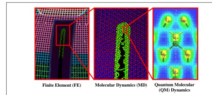
Schematic of hybrid multiscale finite element/molecular dynamics/quantum mechanical simulation of fracture. Continuum FE simulation invokes MD simulation near the crack tip and fractured surfaces to describe atomistic processes, which in turn invokes QM simulation at the crack tip to handle bond breakage/formation and chemical reactions involving environmental molecules (images courtesy of P. Vashishta, University of Southern California).
