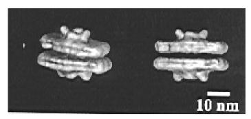
The three-dimensional structure of a plant photo system super complex is reconstructed with sub-nanometer resolution using transmission electron microscopy (image adapted from Nield et al.; reprinted with permission from Nat. Struct. Biol. 7, 44. © 2000, Nature Publishing Group).
