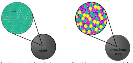
The atoms in stainless steel are arranged in an ordered structure.
