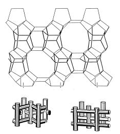
Figure 1. Schematic of the three dimensional channel structure of ZSM-5
