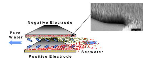
High surface area, high-conductivity electrodes from aligned carbon nanotubes (after Biosource Inc., Sabres of Texas and Boston College)
