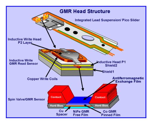
Commercial IBM giant magnetoresistance read head.
