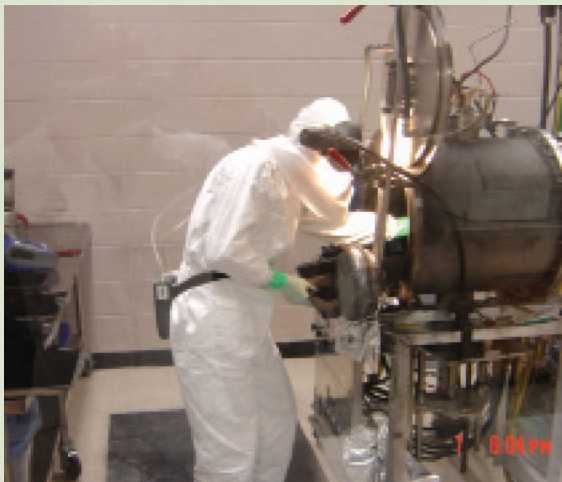
Figure 7. (Left) A researcher harvests single-walled carbon nanotubes from a carbon arc reactor. (Right) An air sample that was collected from the researcher's personal breathing zone (PBZ) while harvesting carbon nanotubes. The image was generated by transmission electron microscopy (TEM) with energy dispersive spectroscopy (EDS).
